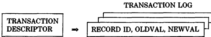
Figure 7. Logical transition logging as implemented in System R. (From Gray et al. [1981].)
